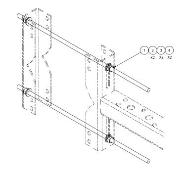
**TOLERANCE NOTES** TOLERANCES ON DIMENSIONS, UNLESS OTHERWISE NOTED ARE: SAWED, SHEARED AND GAS CUT EDGES (± 0.030") DRILLED AND GAS CUT HOLES (± 0.030") - NO CONING OF HOLES LASER CUT EDGES AND HOLES (± 0.010") - NO CONING OF HOLES DESIDE BENDS ARE ± 1/2 DEGREE ALL OTHER MACHINING (± 0.030") ALL OTHER ASSEMBLY (± 0.060")
